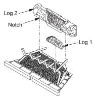
Figure 25 - Installing Logs 1 and 2
